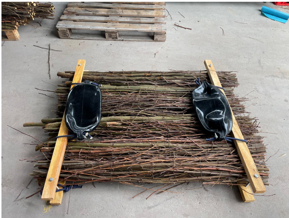
Fig. 2. Finished raft construction with two buoys (source: H2O SCITECH)
