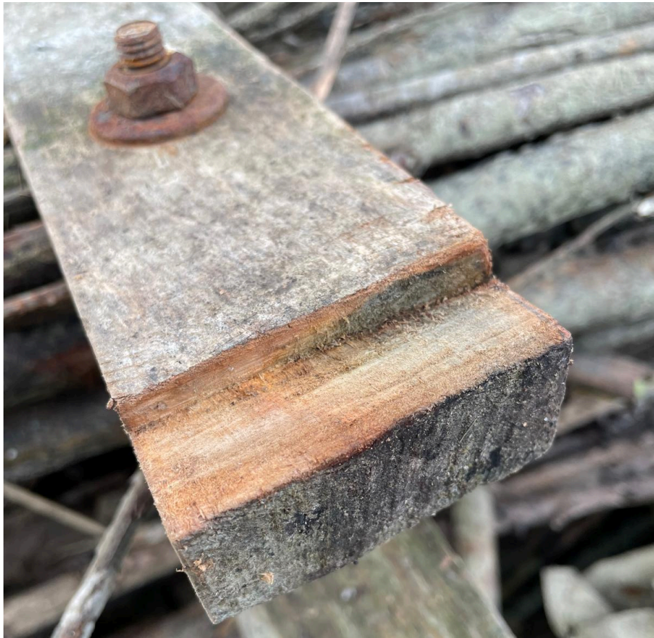
Fig. 17. The condition of the alder wood and screws after the collection of the islands (source: H2O SCITECH)
