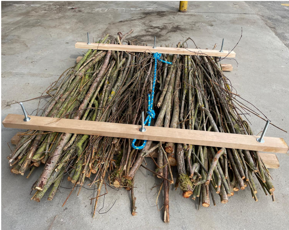
Fig. 2. Prototype raft – element of the plant filter island (source: H2O SCITECH)
